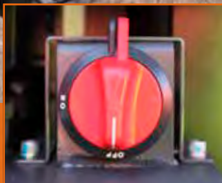
Battery cut-off switch
